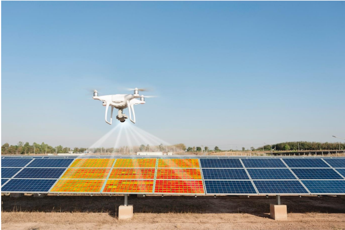
Figure 10. A stylized image showing aerial IR imaging conducted by a consumer drone
