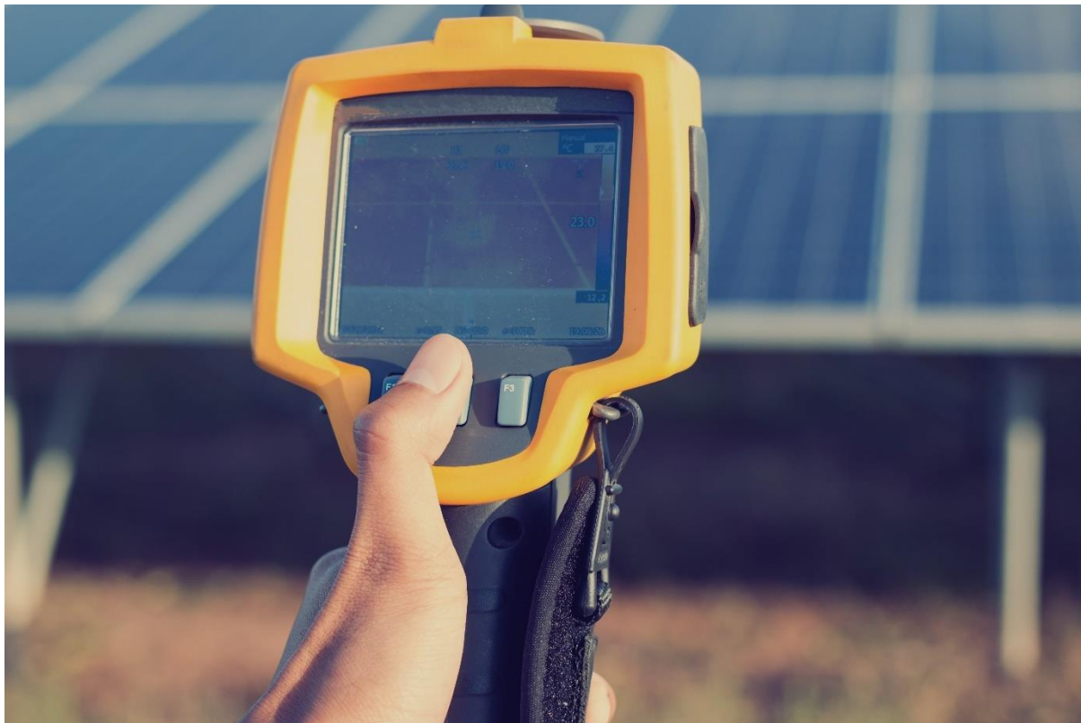
Figure 8. Photo showing field personnel taking an IR image of a solar PV array
